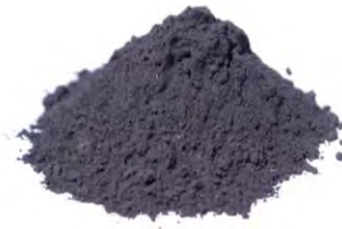
Figure 2: Sample of magnetite material used with the BioMag system.
